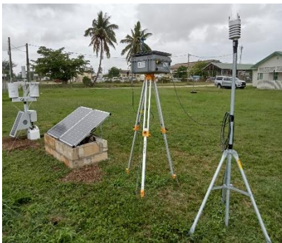
Figure 1: Air Quality Monitoring Station in Tonga urban
